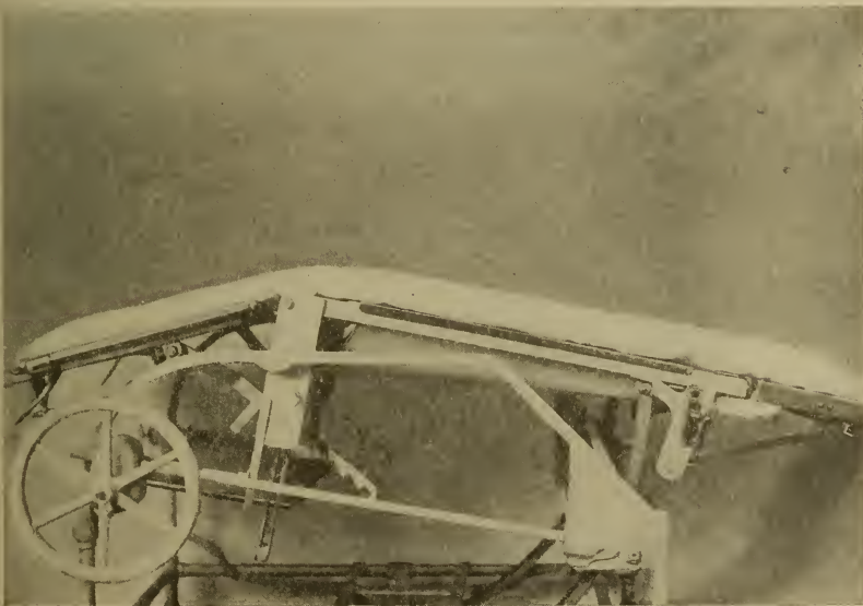
FIG. 31.—Table broken instead of raising rack.
